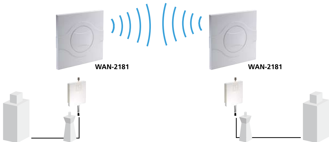
WAN-2181 works with WAB-7000 for Point-to-Point wireless bridging applications
